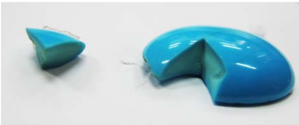
图 5 Zachery 处理绿松石颜色的内外差异 Fig. 5 Different colors of internal part and external part of Zachery-treated turquoise
