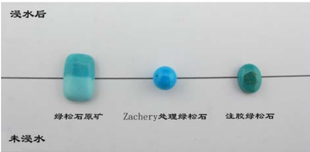
图 6 Zachery 处理绿松石浸水后的颜色变化 Fig. 6 Change of the color of Zachery-treated turquoise after flooding
